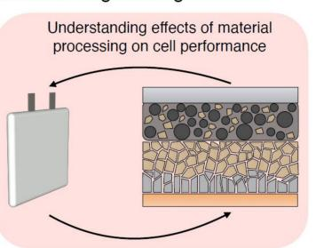
Above: The Chang lab at Drexel University conducts research on batteries and electrochemical engineering, seeking to understand how local material properties (e.g., electrode microstructure and surface chemistry, electrolyte conductivity) affect cell-level behavior (e.g., cycling performance and dynamics, gas formation, changes in mechanical stiffness). Schematic courtesy of Wes Chang, PhD.
